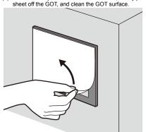
(2) Peel the release paper off the back of the new protective Without peeling off the protective film on the sheet surface.
